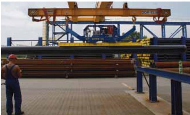
Figure 2. ELiTE 5TD/CD2 – crane double hook application.
