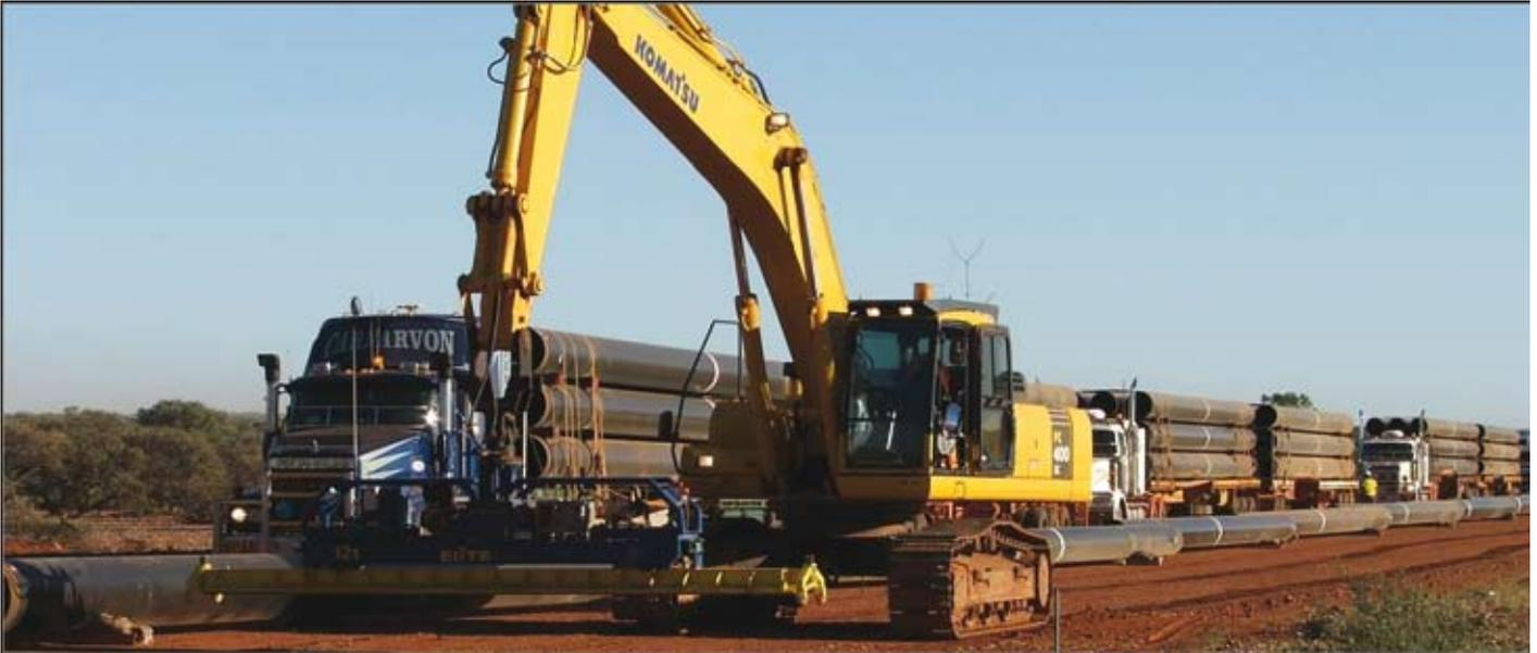
The option of wireless remote controls provides the users with total freedom when handling and operating their vacuum pipe lifters. From this, the operator can easily power up/down the machine and activate/deactivate the suction of a pipe.
