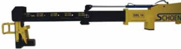
Figure 3. The outer 'stationary' telescope arms are pre-set to lift a particular range of pipe lengths.
